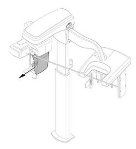
To allow the CS 8100 3D to acquire cephalometric images, we have introduced a sliding mechanism that prevents the X-ray beam from hitting the panoramic / 3D sensor during a cephalometric exam.
